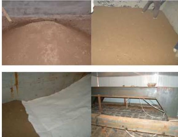
Fig. 3. Process of constructing the channel slope model
